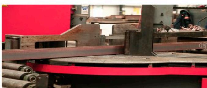
\*The workpiece in the bandsaw is lifted up by 10 mm by hydraulic platforms placed at the entrance and exit of the saw for easy and fast turning of the saw body.
